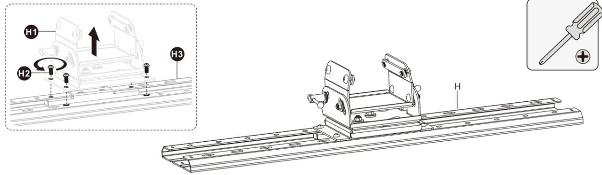
Loosen the screws to leave a gap over 4mm.
