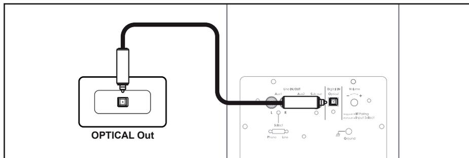
To use the «optical» input to connect our digital devices with help to optical cable. You can get a better audio quality with this input.
