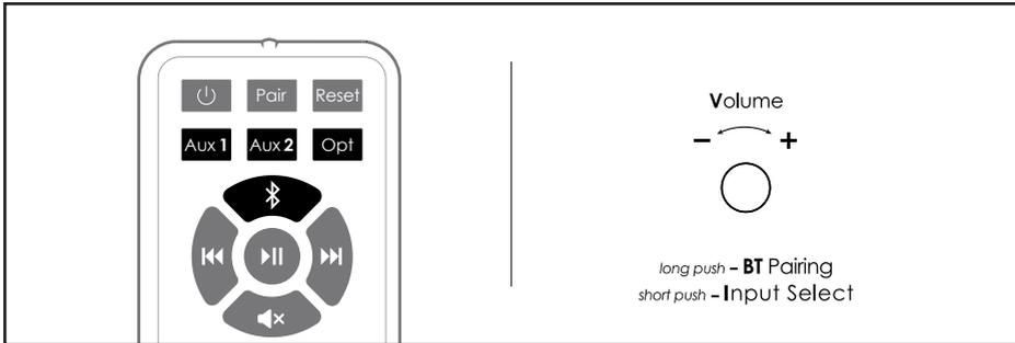
Inputs or sources can be selected with the supplied remote control or with the «Volume Adjustment» on the back of the speaker.
