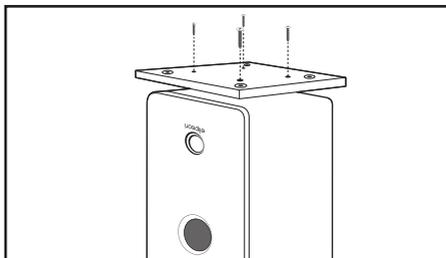
Carefully turn the cabinet over and place it on the packaging foams, or on a carpet, to avoid any damage of the top part. Take care not to damage the woodworking, the lacquered front or the loudspeakers during this operation. Adjust the base on the cabinet and screw it using the four provided screws.
