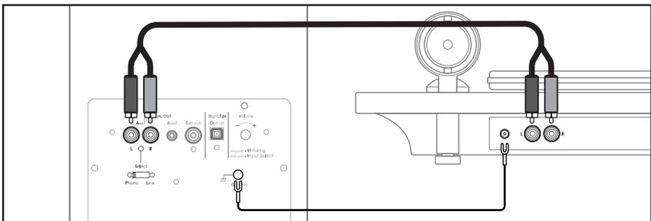
Connect your turntable to the RCA - AUX.1 input. Make sure that the phono or line input selector is in «PHONO» position.
