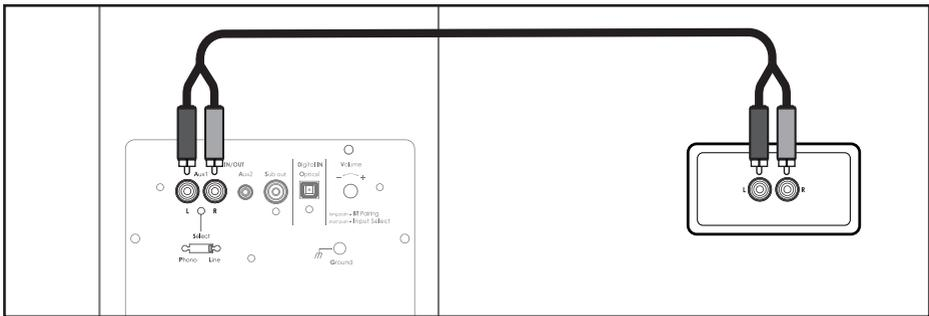
Connect any audio analog stereo source with RCA cable.
