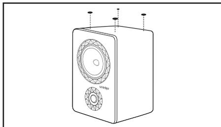
We recommend that you stick the rubber pads, provided with the removable base, on the loudspeakers. If you use the loudspeakers without the removable base, you should place the rubber pads on the provided inserts, to avoid any damage.
