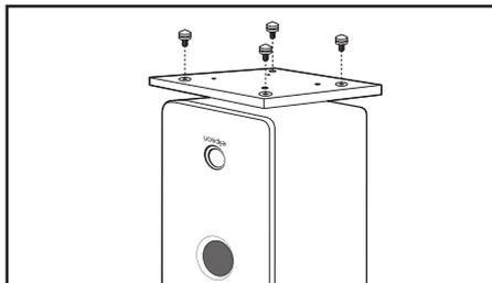
After mounting the base of the speaker, screw the spikes on it (no required tools).
