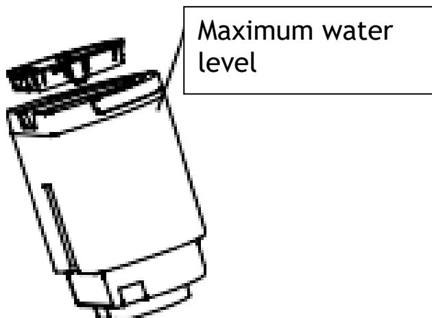
3. Install the clean water tank in the body.
