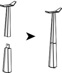
Step 3: Insert the headset stand into the slot on the charging station.
