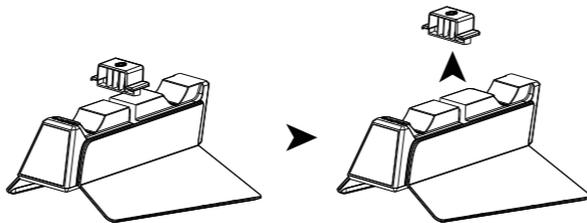
Step 2: Assemble the top and the bottom part of the hanger together
