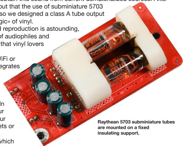
Raytheon 5703 subminiature tubes are mounted on a fixed insulating support.
