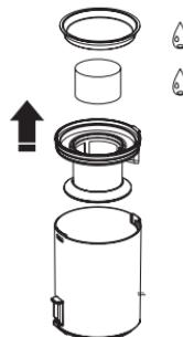
Clean the filter with clean water or a little neutral detergent by rubbing it lightly. Wait at least 24 hours until the filter is completely dry before reinstalling it in the collector.
