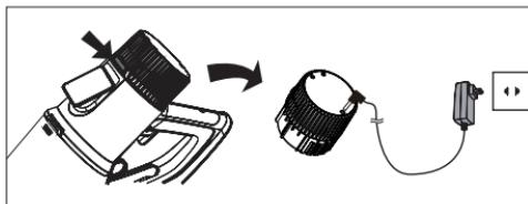
A/ Remove the battery from your device and plug the AC adapter directly into the battery.
