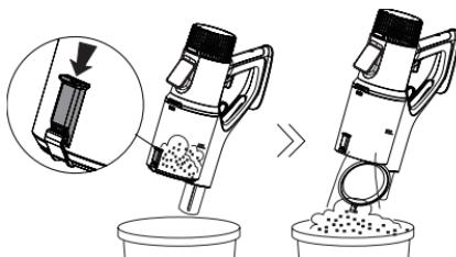
Press the button on the manifold to open and empty it.
