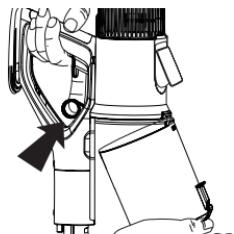
It is also possible to remove the collector by pulling the ring to completely empty and clean it.
