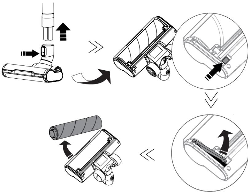
Once the brush has been removed from its block, use a sharp object to remove the bristles and coiled hair. The brush can be rinsed under clean water to clean it. Just be sure to let it dry for 24 hours for 24 hours and ensure that it is completely dry before reinstalling it as follows:
