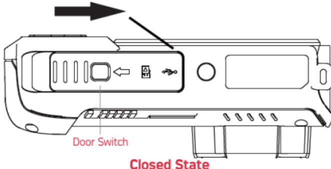
Hold the hatch switch and push the hatch in the direction of the arrow to open it
