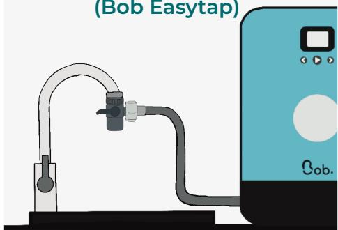
Via a Bob Easywater water inlet hose or equivalent, the tank will be filled automatically at the start of each cycle.
