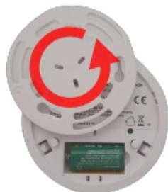
**CHARACTERISTICS:** Powered by 1 DC3V CR123A / CR17335 battery • Battery life up to 5 years • Max product lifespan: 10 years. Beyond that, the device must be replaced even if it is still functional • Photoelectric sensor • Requires a 2.4Ghz WiFi network b/g/n • Red LED alarm indicator • Alarm sound level approx. 85dB at 3 meters • Operating conditions: temperature between 0°C and 50°C, max humidity 95% • Low battery warning • Dimensions: 31 mm thick, 86 mm in diameter
