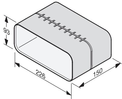
DFK-L Length adjustment 150 mm, Installation drawings
