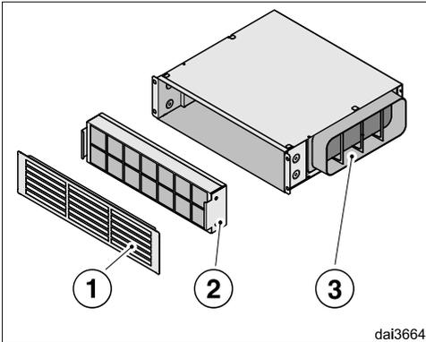
Air is drawn in and passed through a grease filter in the cooker hood to clean it. It is then directed into the recirculation box where it passes through a reactivatable charcoal filter ② where it undergoes further cleaning before being directed through a ventilation grille ① back into the kitchen.
