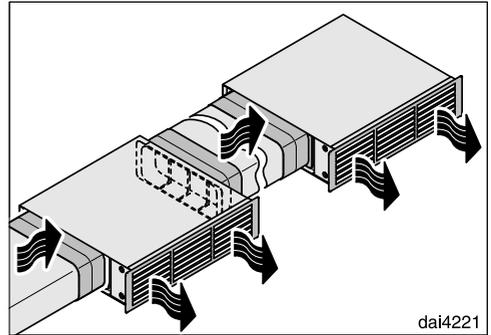
You can connect multiple recirculation boxes to one another. This improves odour reduction performance, boosts the air flow rate, and results in a lower flow velocity at the recirculation grilles.
