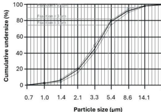
Measurements were performed using a salbutamol solution with a "Next Generation Impactor" (NGI). The diagram may therefore not be applicable to suspensions or highly viscous medications. You can obtain more detailed information from the manufacturer of your medication.
