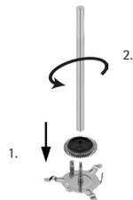
To reassemble, push the milk DISC (9) into the DISC bracket (8) with the notch facing upwards. Then screw the handle (7) all the way into the DISC bracket (8) from above. The milk DISC (9) is now affixed flexibly to the bracket.
