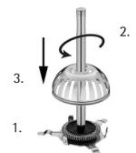
To reassemble the WMF Choc System, push the milk DISC (9) into the DISC bracket (8). Then screw the handle (7) all the way into the DISC bracket (8) from above. The milk DISC (9) is now affixed flexibly to the bracket. Next push the chocolate basket (10) onto the handle (7) from above and push downwards until it clicks into place.
