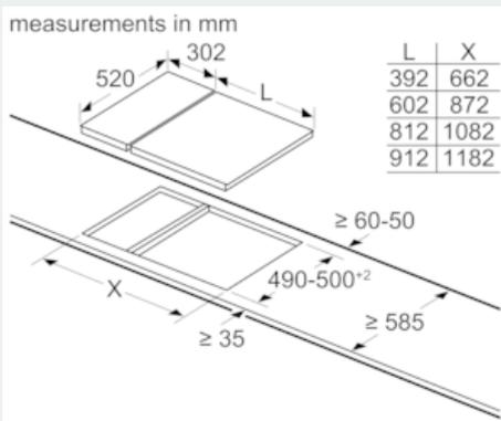
When installing a Domino unit right next to a hob, an assembly kit (HZ394301) is required.
