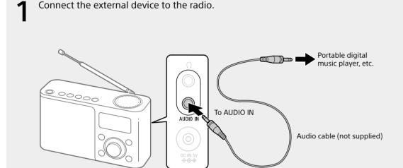
When connecting an external device to the unit, use audio cable with a stereo (3-pole) or monaural (2-pole) mini plug. If you use another type of plug, there may be noise interference or no Compatible plug types Other types of plugs cannot 3 or more rings
