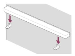
Align the positions of the screw holes on the bottom of the bar speaker and holes of the wall mounting bracket, then fix the bar speaker to the wall mounting brackets by fastening the screws (supplied) securely.
