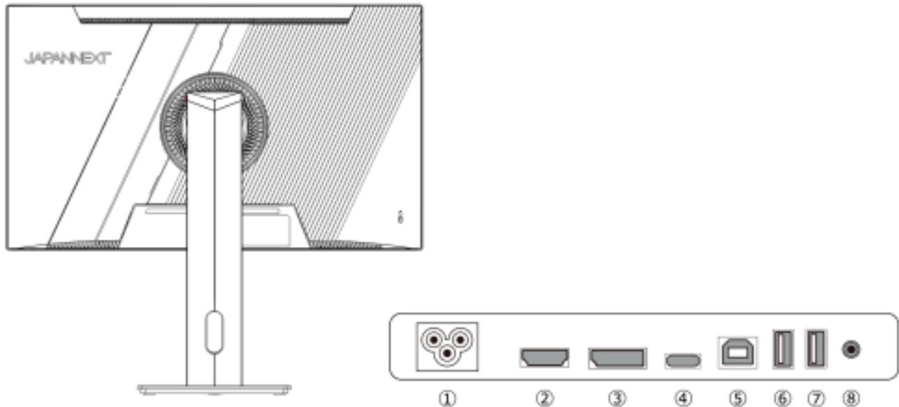
**1: Power supply:** Used when connecting the power cable.
