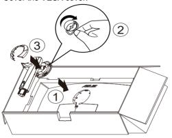
4. Fix the base to the arm by fastening the bundled screw.
