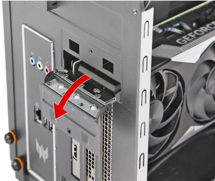
4. Detach the graphics card from the PCIe x16 extension slot.
