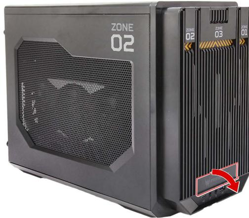
2. Pull out the portable SSD device from the chassis.
