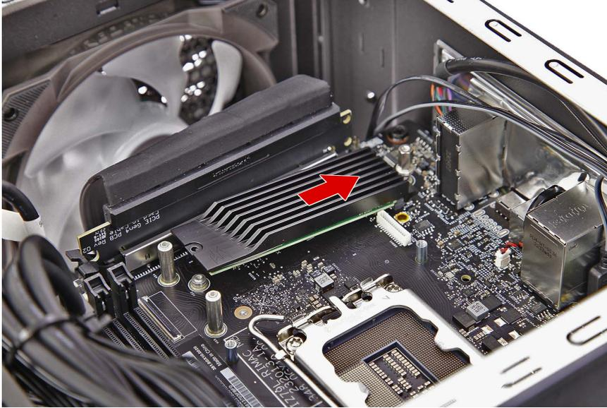
4. Secure the SSD1 module to the mainboard using one screw.
