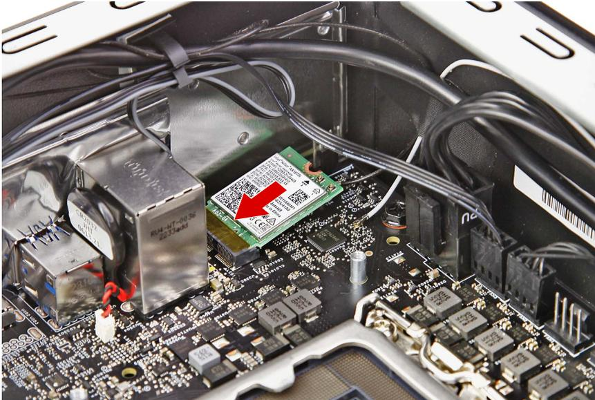
2. Secure the WLAN module to the mainboard using one screw.
