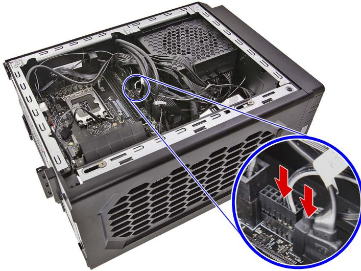
6. Secure the cables to the chassis using the cable tie and plastic clips.
