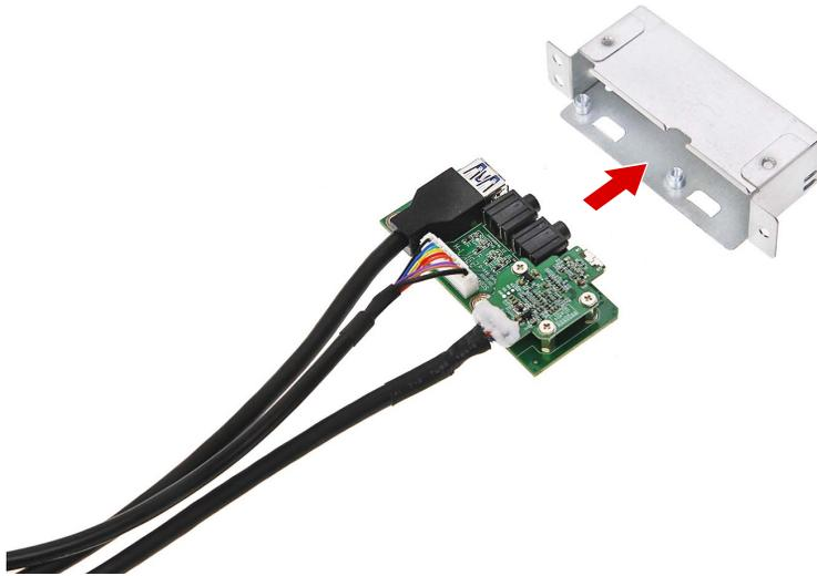
2. Secure the front I/O board to the bracket using two screws.
