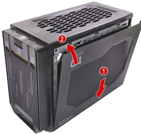
2. Secure the right side panel to the chassis using two screws.
