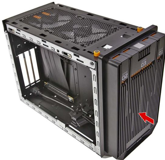
3. Secure the front bezel to the chassis using four screws.
