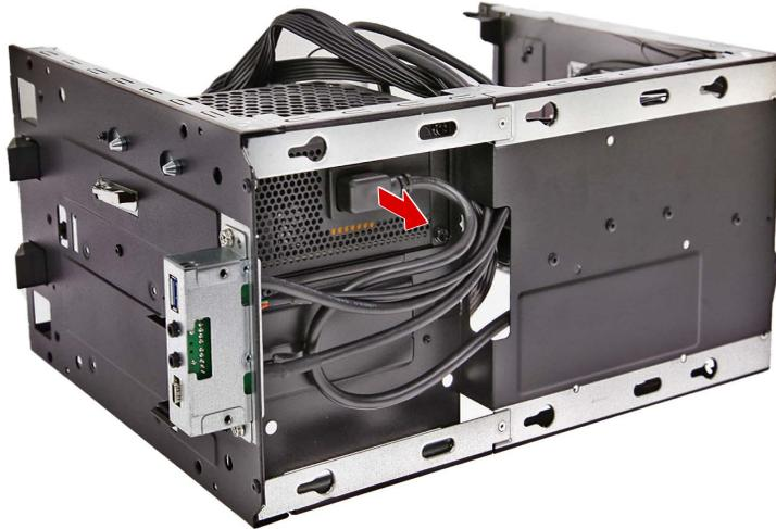
2. Disconnect the power supply cables from the mainboard.
