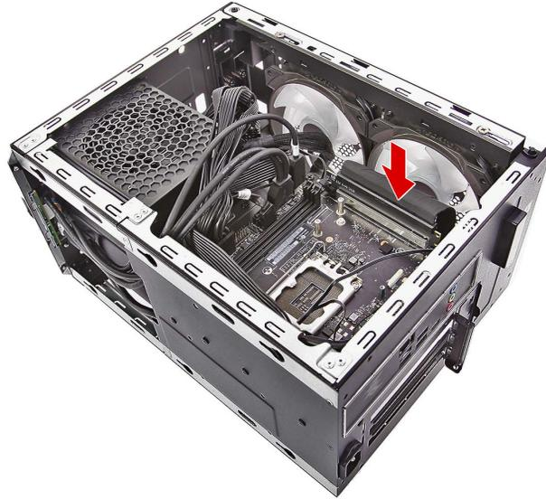
4. Secure the PCIe x16 extension cable using adhesive tape.
