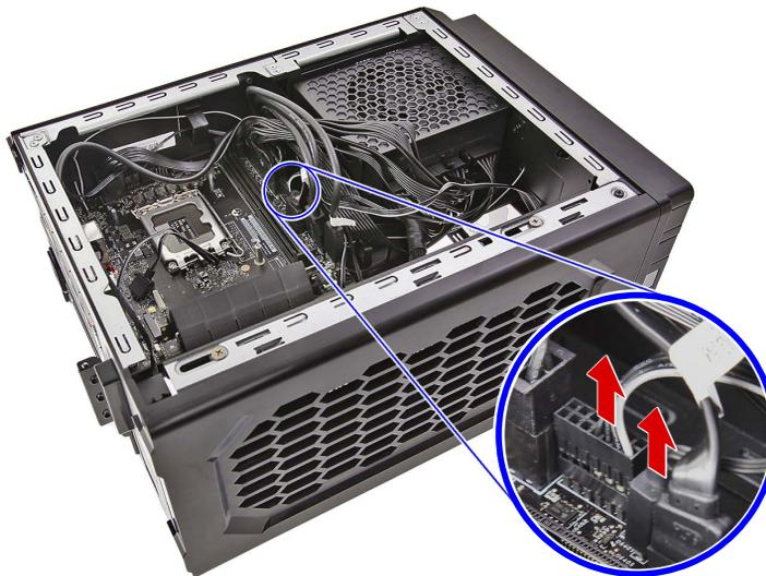
3. Release the power button/LED cables from the metal clip that secures them to the chassis.
