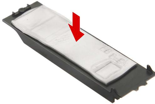
2. Insert the SSD2 module into the SSD heatsink.
