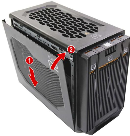
2. Secure the left side panel to the chassis using two screws.
