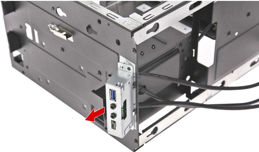
5. Pull out the front I/O and audio cables from the chassis.
