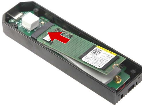
3. Secure the SSD module to the portable SSD device using one screw.
