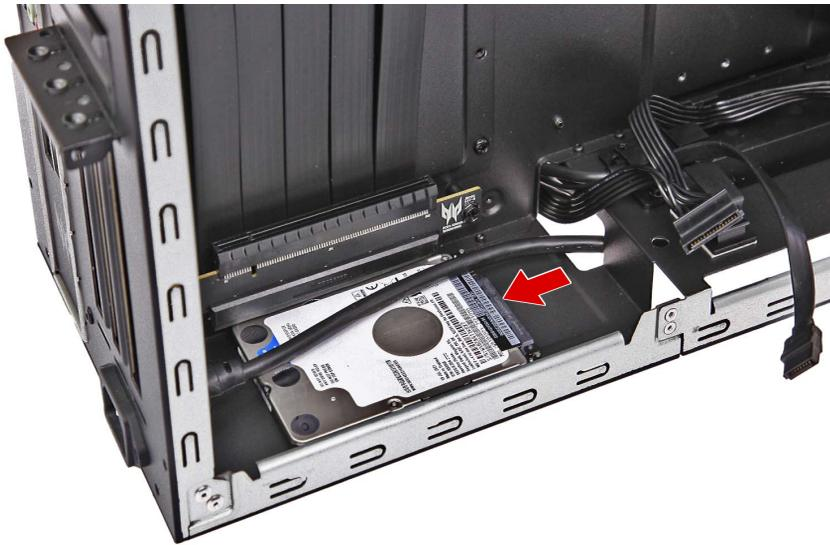
2. Secure the HDD2 module to the chassis using four screws.
