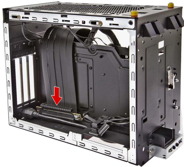
2. Secure the PCIe x16 extension cable to the chassis using two screws.
