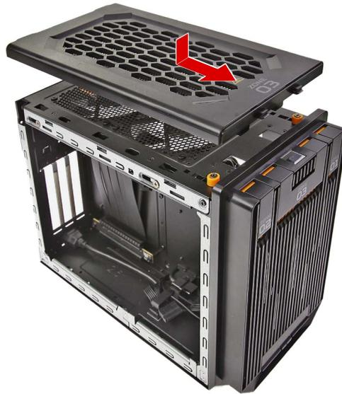
2. Secure the top cover to the chassis using two screws.
