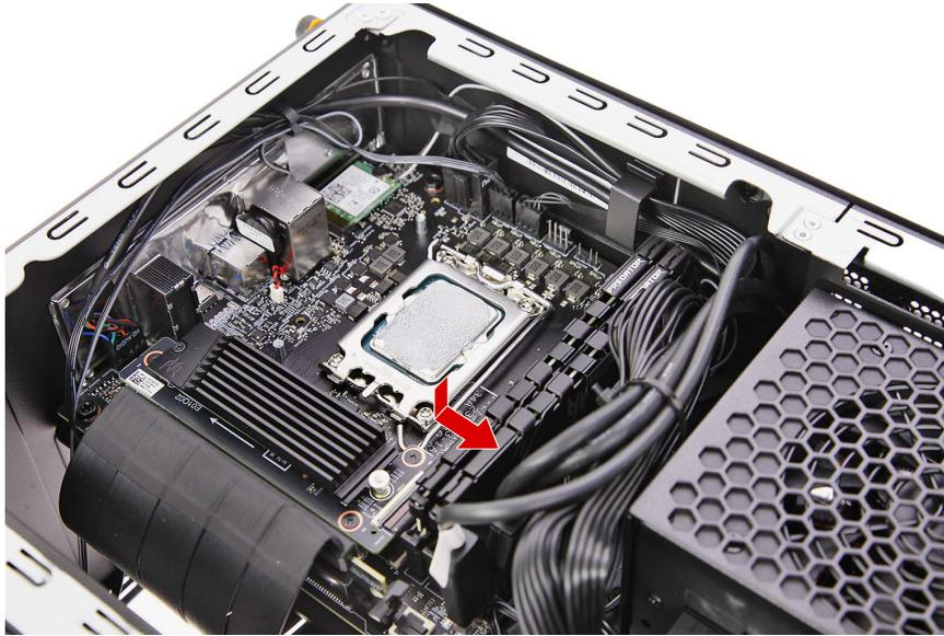
2. Pull the load lever to release the processor from its socket.
