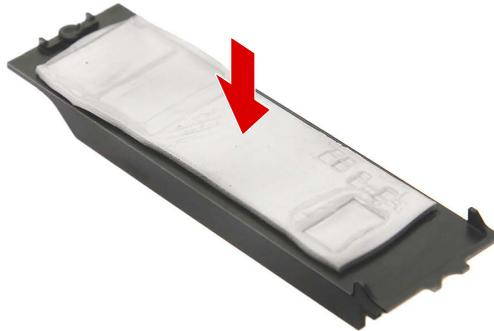
2. Insert the SSD1 module into the SSD heatsink.
