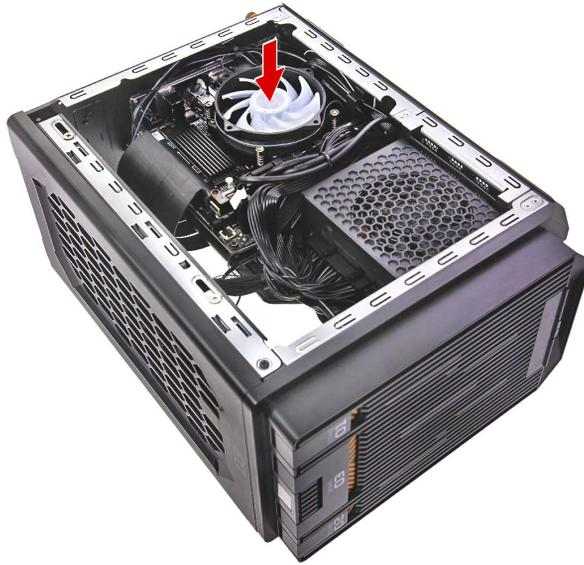
2. Tighten the four captive screws to secure the thermal module to the mainboard.
