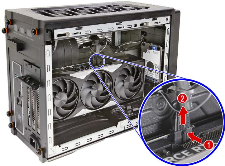
2. Remove the three screws securing the graphics card brackets to the chassis.
