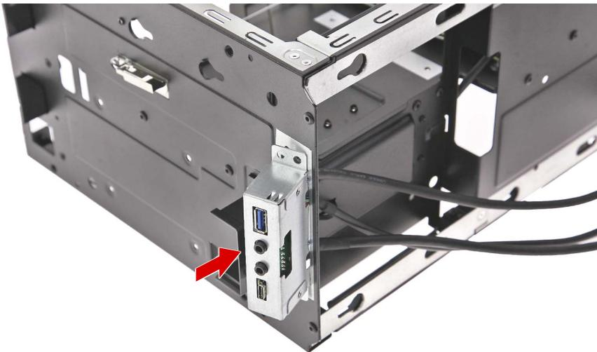
5. Secure the front I/O bracket to the chassis using two screws.
