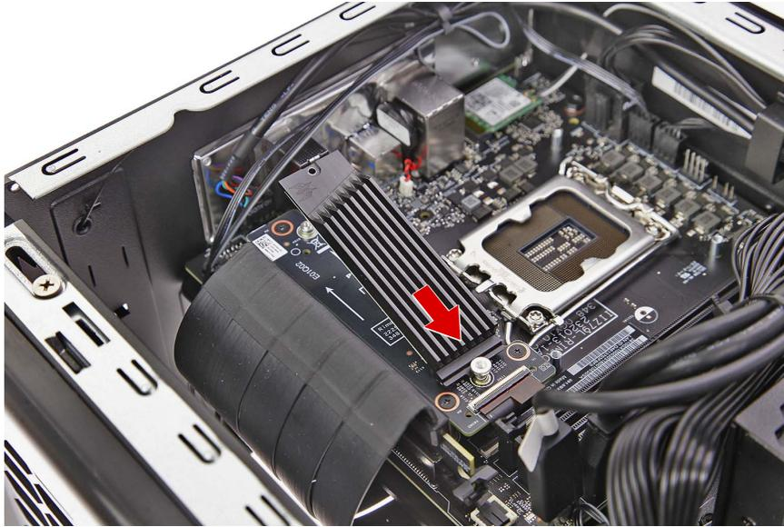
4. Secure the SSD2 module to the mainboard using one screw.
