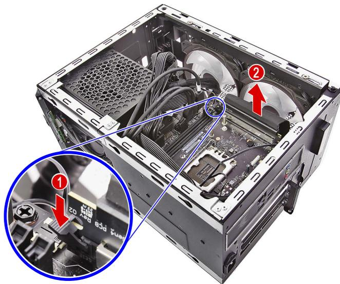
3. Remove the two screws securing the PCIe x16 extension cable to the chassis.
