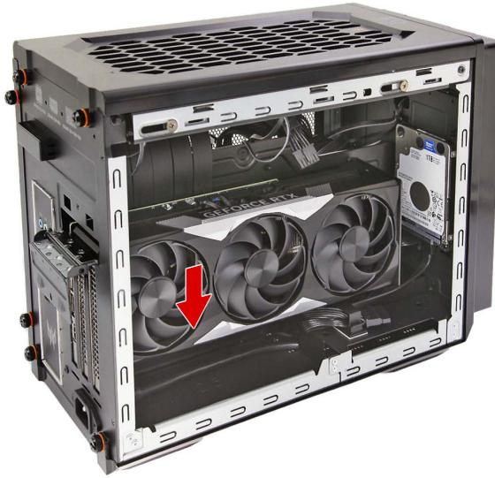
2. Use the metal clip to secure the graphics card bracket to the chassis.
