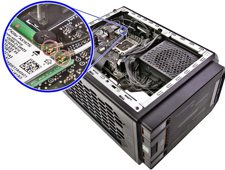
**NOTE:** Refer to your machine disassembly note to determine which cable color corresponds to the main and auxiliary connectors.
