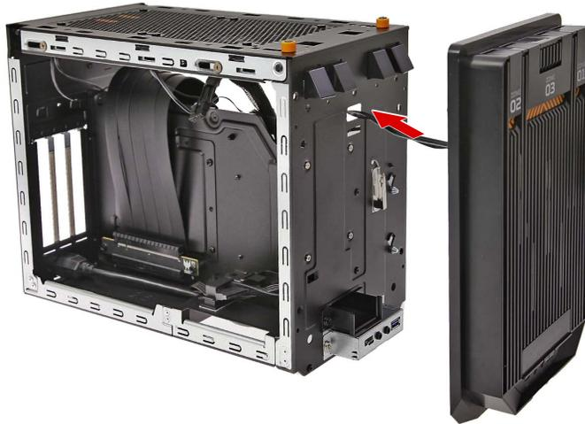
2. Push the front bezel into the chassis until the latches lock into place.
