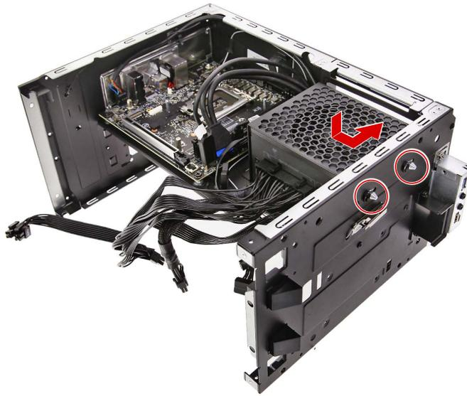
2. Secure the power supply module to the chassis using four screws.
