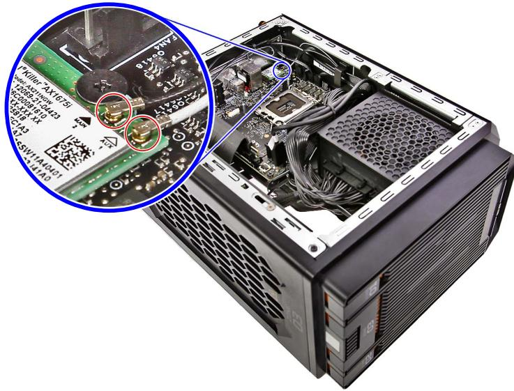
**NOTE:** For reference during machine reassembly, note which cable color corresponds to the main and auxiliary connectors.
