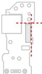
2. Install the I/O board, then fix it with the screws you removed previously.
