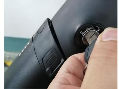
Remove the battery from the frame of the bike.
