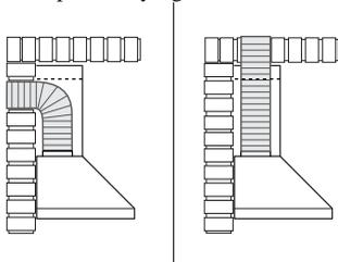
Maximum ducting distance should be 3 meters, with one 90 degree bend.
