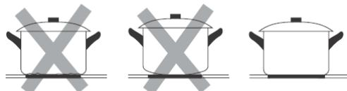
If the base of the cookware is only partially ferromagnetic, only the area that is ferromagnetic will heat up. This may mean that heat will not be distributed evenly. The non-ferromagnetic area may not heat up to a sufficient temperature for cooking.
