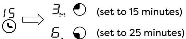
2. Once the countdown timer expires, the corresponding zone will switch off. Then it will show the new min. timer and the dot of corresponding zone will flash.
