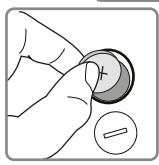
Insert battery with + mark facing up. Lock battery cover into position by turning the cover clockwise.
