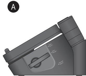
Push Latch into Store position to store.
