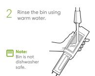
3 Make sure bin is completely dry. Reinsert filter and place bin back in the robot.
