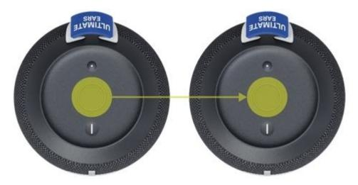
After pairing, LONG-PRESS the center button on either speaker to toggle between the standard mono mode (louder volume) and two-channel stereo mode.
