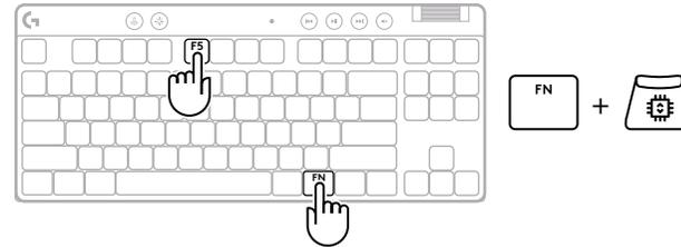
**2** Enter Rapid Trigger adjustment mode.
