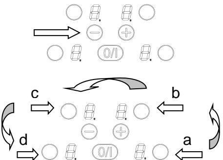
3) Remove your fingers from the touch control, press simultaneously [ + ] and [ - ] during few seconds, until blinking [ E ] symbols appear.
