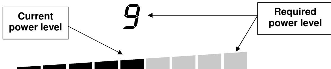
The segments from the power display are turning on one by one until the required power level is reached.
