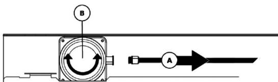
A. First disconnect the cable that runs to the LED to be replaced. Disconnect by loosening the lock by exerting slight pressure while pulling loose.
