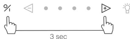
To switch the InTouch function off press the 1 and 2 keys at the same time for 3 seconds and the 2nd and 4th LEDs flash 3 times to confirm. (The appliance must be switched off).
