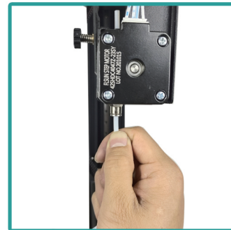
27.Insert the PTFE tube into the extruder until it can no longer forward
