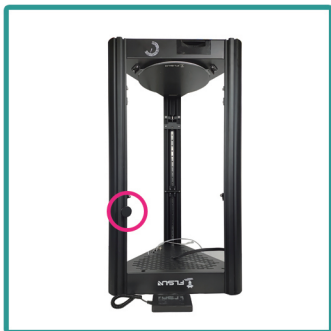
13. Move the touch screen bracket to one-third of the distance from the top case
