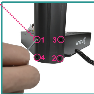
5. Install the screws in the order from 1 to 4
