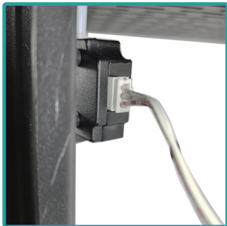
25.Plug the filament detection sensor cable
