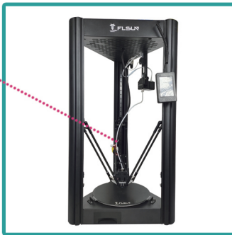
29.Tie the PTFE tube and the main cable together at the location marked in the photo
