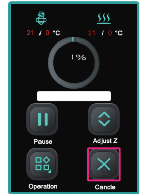
24. Adjust the distance between the nozzle and the hot bed to a proper distance then click "Cancel"
