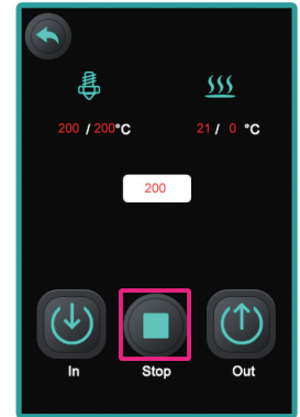
12. When the filament is extruded from the nozzle, click "Stop"
