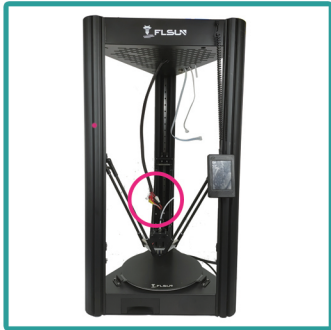
19. Connect the connector of the effector module to the main cable
