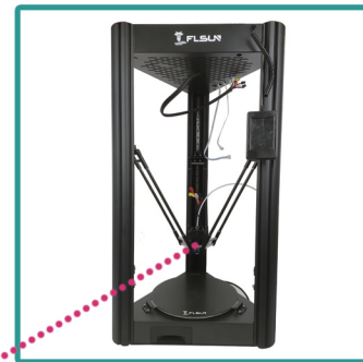
18. Install the effector module the logo on the effector module must face forward
