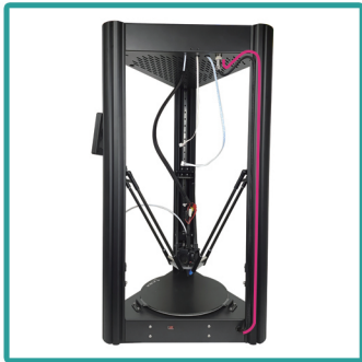
22. Put the right main cable into the groove in the axis
