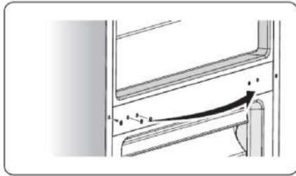
9. Lie the refrigerator backwards, Remove ④ (right), Remove three self-tapping screws from the lower hinge part(right). Loosen the lower hinge axis then install it on the reverse hole site, and tighten into position(change it into left hinge part). Remove the lower hinge part to the left-bottom corner of the cabinet, Then fix it with 3 screws, finally install part ④ on the left-bottom and right-bottom of cabinet.
