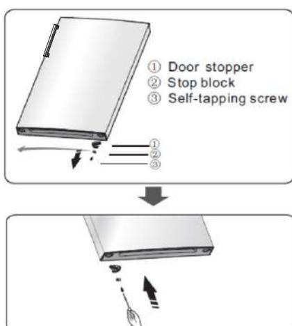
6. Use the Allen wrench(provided in the plastic bag) to loosen screws used to fix the right middle hinge and remove right middle hinge. Then remove the lower door.
