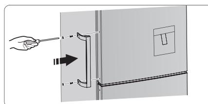
3. Fix the handle with the special screws provided in the plastic bag. And then install the handle covers.
