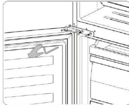
11. Carefully slot the upper door onto the middle hinge pin and hold in position. Move the upper door to an appropriate position, adjust left upper hinge(in the plastic bag) and upper door, then fit the hinge pin into the hinge hole at the top and the door to secure the door in place. Then fix the upper hinge part with screws (Please carefully hold upper door by hand when installing).
