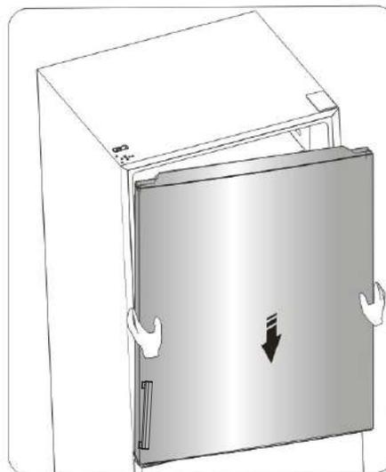
12. Assemble the left hinge cover provided(in the plastic bag) to match the hinge, install the door racks to original position. Keep the right hinge cover with the appliance for future reference.
