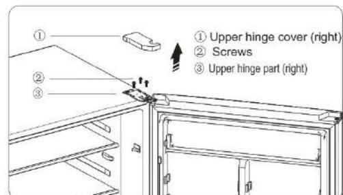
3. Remove screw cover from the left-front corner of cabinet with flat head screwdriver and install screw cover-right to the right front corner. Put the upper
