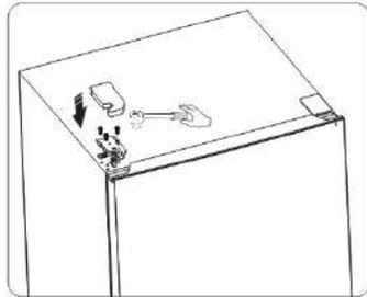
16. Remove the upper door and place it on a smooth surface with its panel upwards. Lever part ① and part ④, then loose screws ②, as shown in the picture. Change handle ③ to the right side, then install screws ②, part ① and part ④ in turn.
