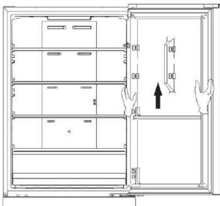
5. Place the upper door on a smooth surface with its panel upwards. Loosen screw ③ and take down part ② and part ①, Install replacement door stopper-left provided (in the plastic bag attached) and left stop block to the left side with screw ③. Conserve part ① and ② with the appliance for future reference.
