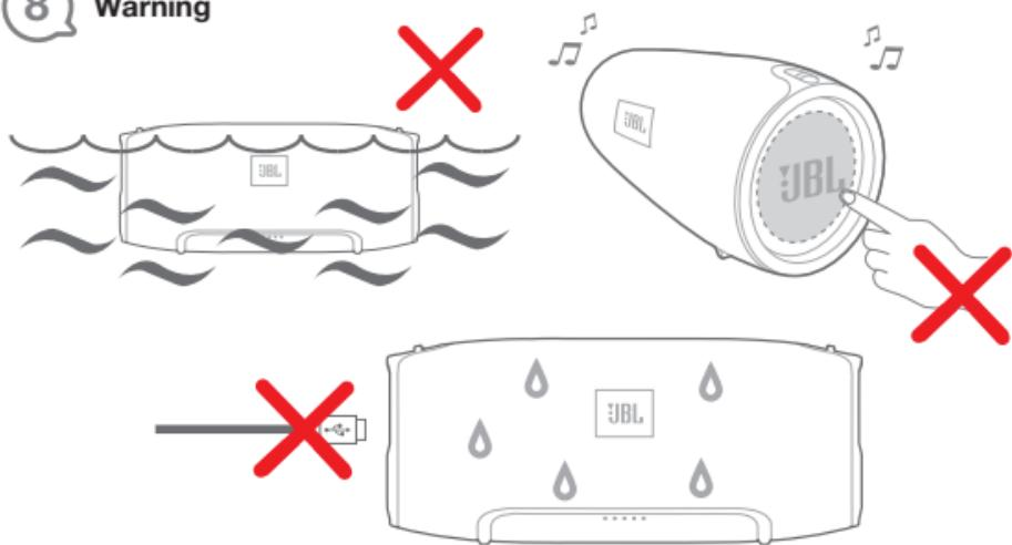
JBL Xtreme is splashproof; submerging it in water or other liquids may result in permanent damage to the speaker.
