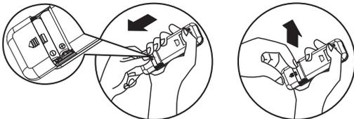
2. Insert new batteries making sure that the (+) and (-) of battery are matched correctly.
