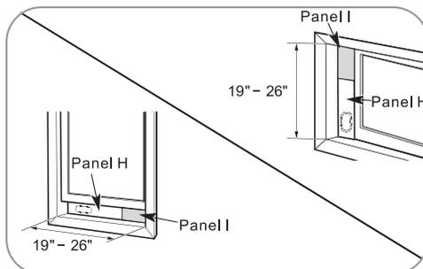
For window openings from 19" to 26", use the window vent panel (Panel H) and an extension panel (Panel I).
