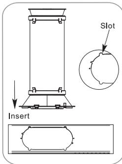
Align the tabs on the window exhaust adapter with the slots in the vent panel. Insert the window exhaust adapter into the opening in the vent panel.
