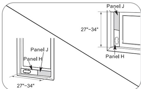
For window openings from 27" to 34", use the window vent panel (Panel H) and an extension panel (Panel J).
