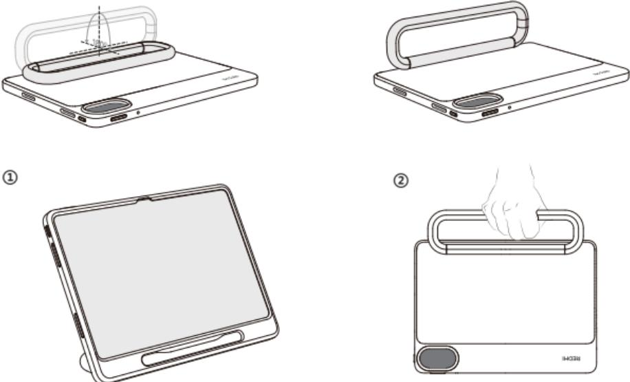
\*Rotate the kickstand ring 180° for hanging or carrying purposes. Avoid excessive swinging while carrying the device by hand to prevent mechanical damage.
