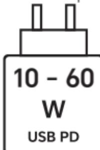
The power delivered by the charger must be between min 10 Watts required by the radio equipment, and max 60 Watts in order to achieve the maximum charging speed. USB PD fast charging.
