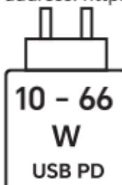
The power delivered by the charger must be between min 10 Watts required by the radio equipment, and max 66 Watts in order to achieve the maximum charging speed. USB PD fast charging.
