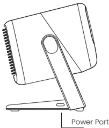
**Power on/off:** The power button is a physical button, short press to power on or off.
