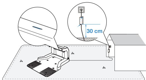
**Note:** Please ensure the power adapter is positioned 30 cm above the ground to prevent water and moisture damage.
