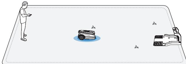
If the base station is not on the lawn, control the ECOVACS GOAT to move to the lawn boundary, then start Mapping.
