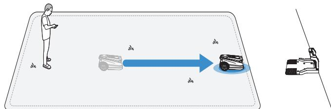
**Note:** To ensure successful recharging, it's recommended to keep the base station within 3 meters of the lawn, and no more than 10 meters away.
