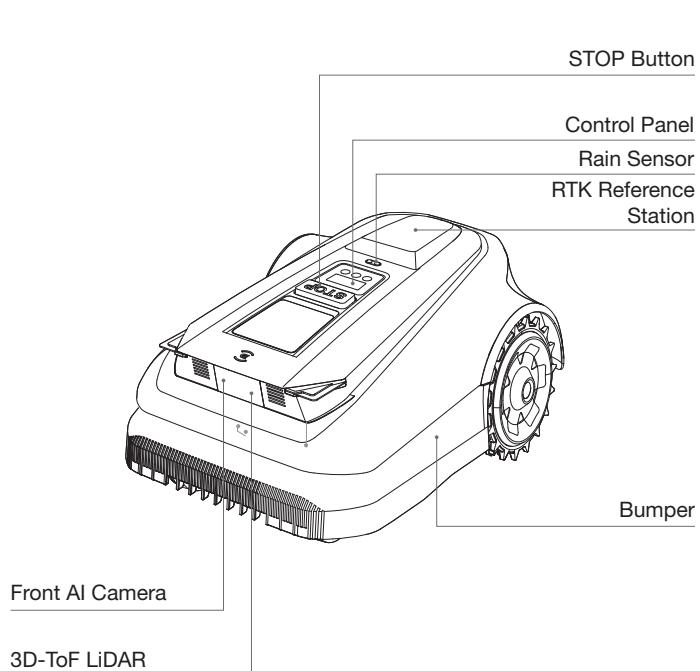
**Control Panel:** The buttons on the control panel can be used for the basic operations of the mower. The digital numbers on the dashboard display shows mowing progress, battery level, and mower status.
