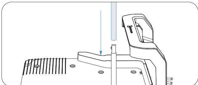
2. Insert the triangular peg into the mounting pole and tighten it securely.
