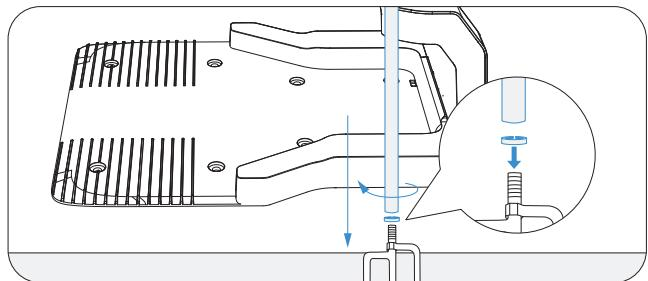
3. Attach the signal head by inserting its raised part into the mounting pole and tightening the screws with a tool.
