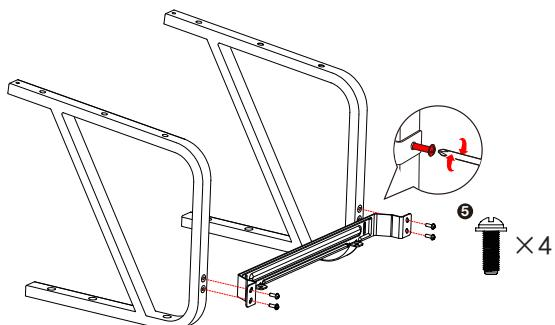
**② Insert the rod into each of the left and right braces separately.**
