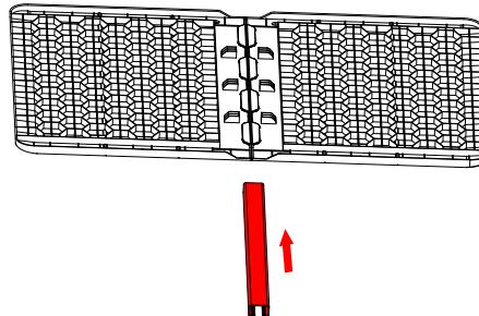
**5 Place the sunshade panel upside down on the frame and secure it with interlocking screws.**
