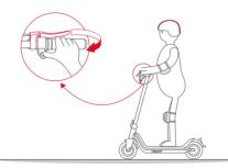
Release the throttle twistgrip and use the energy recovery to achieve the effect of deceleration. Emergency braking requires powerful grip on both sides of the brake levers. \*The deceleration can be adjusted through energy recovery within the App.
