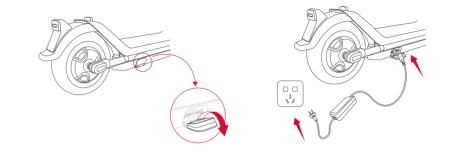
Firstly open the charging port, then plug the charging plug into the body charging port and finally connect the power supply to charge. After the completion of charging, fastening down the charging port to beware of water intake.
