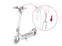
Lock the screws on both sides alternately with the hexagon wrench in the packaging box (tightening torque: 4~5N\*m), that is, the assembly is completed.
