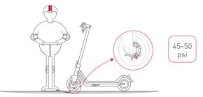
If your kick scooter front and rear tires are underinflated, please use the extension nozzle to connect the car body tires to inflate. First remove the front and rear tire inflatable nozzle cap, and then tighten the extended inflatable nozzle and tire inflatable nozzle, and connect the pump to inflate after they are to be tightened.
