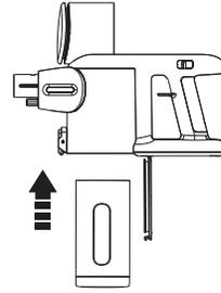
Insert the multi-cone assembly removal tool upwards into the dustbin.
