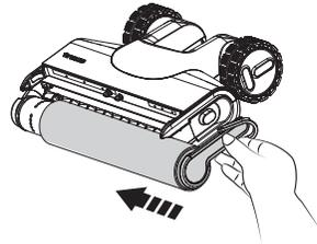
Replace the brush roller by inserting its end into the left side of the holder, then attach the roller tab to the magnetic buckle on the right side to lock into place.
