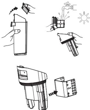
Grasp recessed area on each side of the dry filter and pull upward. Rinse under running water and must be completely dry before recombining with the lid of the DWT.
