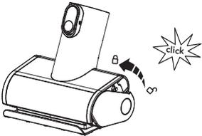
Fully reinsert the brush roller at an angle and push upward until it clicks securely back into place.
