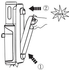
Place the tank back into the appliance. You should hear a "click" if done correctly.
