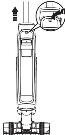
To remove the handle, press the release button on the back of the appliance, then pull the handle upwards.
