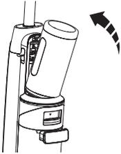
To install, insert the SwitchPro Motor into the floor washer, push it in, installation is complete when you hear a click.
