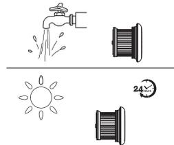
The HEPA filter can be washed under running water and must be completely dry before reinstalling.
