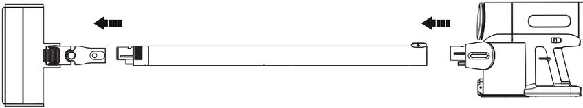
Connect the brush, tube and main body as shown above.
