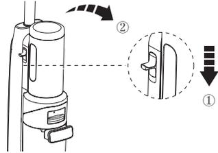
To remove the SwitchPro Motor, hold the appliance with one hand and press the release slider with the other hand.
