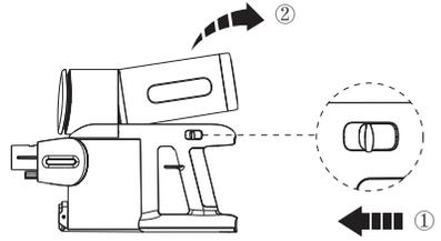
To remove the SwitchPro Motor, hold the appliance with one hand and press the release slider with the other hand.
