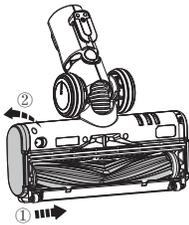
Fully reinsert the brush roller into the brush window and the end cover can be rotated counter-clockwise until it clicks securely back into place.
