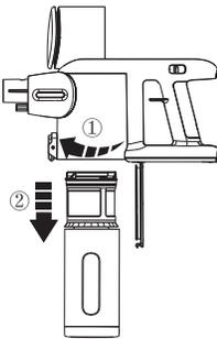
Rotate to remove the mesh filter.
