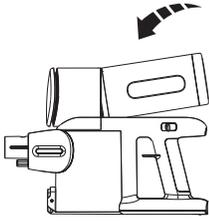
To install, insert the SwitchPro Motor into the vacuum cleaner, push it in, installation is complete when you hear a click.
