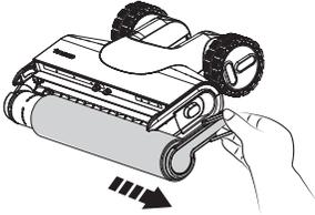
Remove the brush roller by grabbing the brush roller tab and pulling out.
