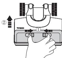
Squeeze latches on the cover and pull upward to remove.
