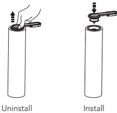
Pull up the roller handle to remove it. Once removed, install the handle into the new brush roller.
