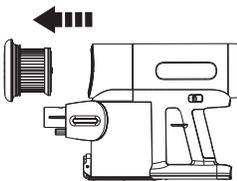
Pull out the HEPA filter (in magnetic design) for cleaning. Do not use the appliance without first installing the HEPA filter.
