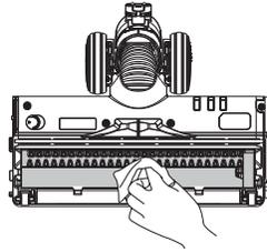
Slide the switch to open the brush roller end cover, and rotate it clockwise before pulling out the brush roller.
