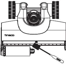
Remove hair and debris from the brush roller chamber and the opening with the cleaning tool.
