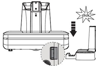
Insert the drying & charging dock into the vacuum dock as shown. Installation is complete when you hear a "click."
