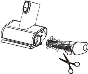
Remove the debris wrapped around the roller with a cleaning tool.
