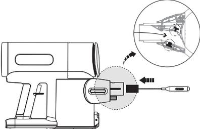
To avoid dust accumulation which can affect cleaning performance, wipe the suction mouth with the cleaning tool.
