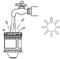
Clean the filter and dry it completely before reinstalling.
