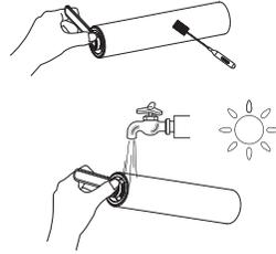
Use the cleaning tool to remove the hair and debris wrapped around the roller and rinse the roller with water, and allow it to dry completely before reinstalling.
