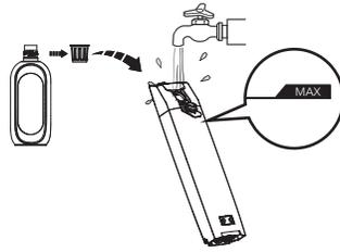
Open the tank cap, and fill the tank with tap water to the Max line. When deep cleaning is necessary, add one bottle cap of solution to the CWT and tightly close the cap.
