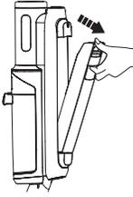
Press the Clean Water Tank release button to remove CWT from the appliance.
