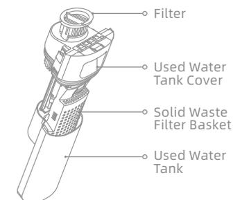
3. Rinse the Used Water Tank, including the separation motor on the tank cover, solid waste filter basket and tank cover with water. Use the provided cleaning brush to clean the inner walls of the tank.
