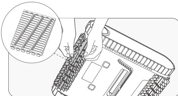
2. Once removed, take the replacement roller brush and align the silicone buckles with the slots. Press the buckles into each slot to secure the new roller brush to your device. Repeat this step for the other roller brush.
