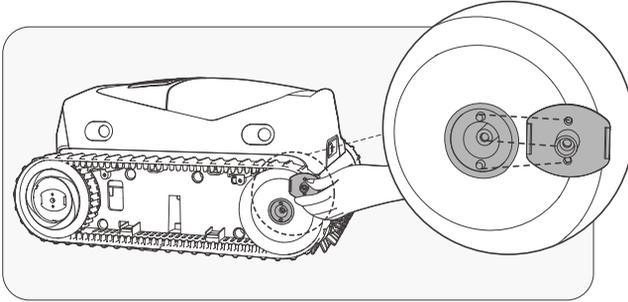
6. Tighten the screws and reinstall the side cover plate. Repeat this step for the other caterpillar tread.
