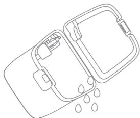
2. Rinse the used water tank with clean water, and use a proper cleaning tool to clean the inner wall of the used water tank.
