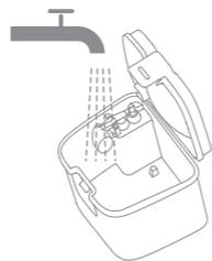
**Note:** The float ball in the used water tank is a movable part. Do not apply too much force when cleaning it to avoid damaging it.
