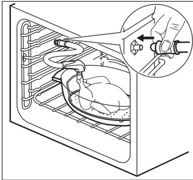
2. Put the baking dish onto the first or second shelf position from the bottom.
