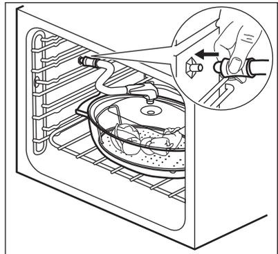
Make sure that you do not crush the injector tube or let it touch a heating element on the top of the oven.
