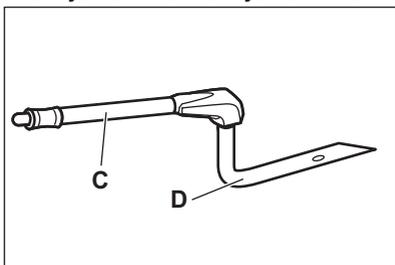
"C" is the injector tube for steam cooking, "D" is the injector for direct steam cooking.
