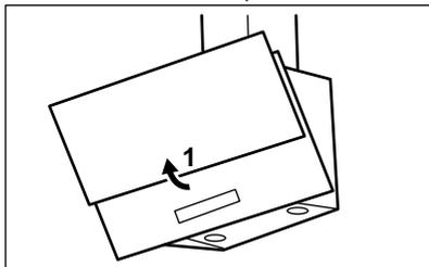
2. Press the handle of the mounting clip on the filter panel underneath the hood (1).
